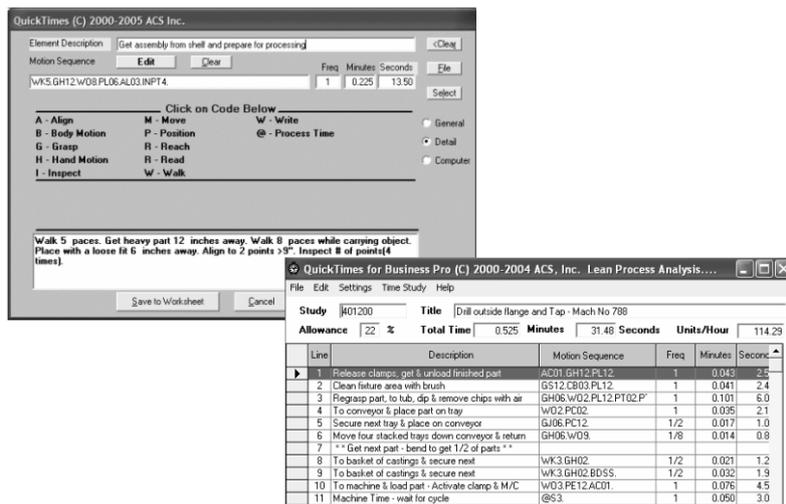
Fig. 3. Generation of the descriptive sentences for the activity, standardization sheet in the Quick Times mode
