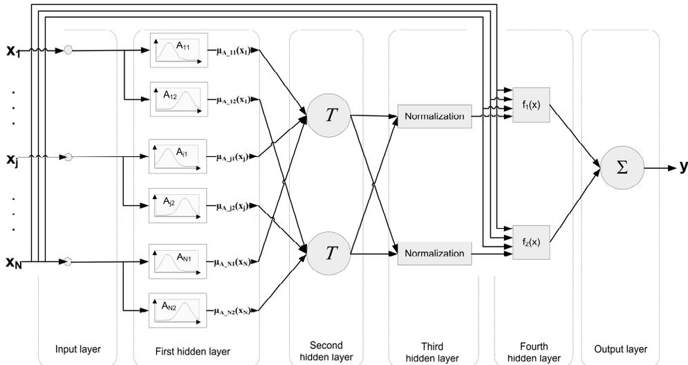
Fig. 1. The ANFIS system which reflects inference of the TSK model with  $N$  inputs, one output and two conditional rules
