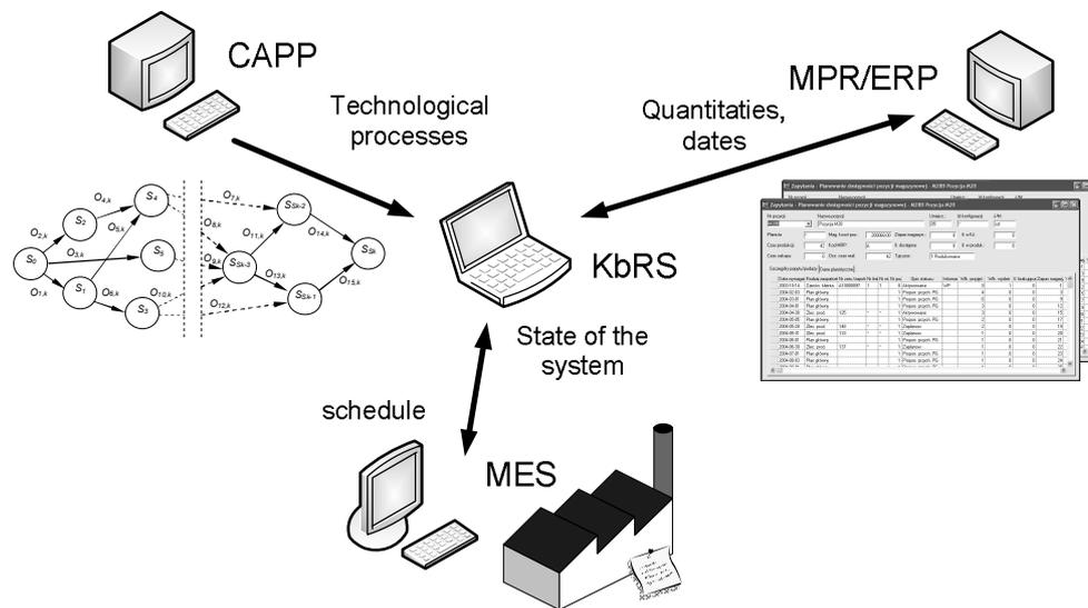
Fig. 1. The KbRS interaction with other production IT systems [18]
