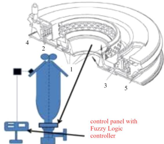
Fig. 3. Segment cooling ring with automatic regulation of film-cooling airflow: 1 – dual-flow cooling ring, 2 – adjusting actuators, 3 – actuator unit, 4 – actuator positioning drive, 5 – perimetric air inlet; arrows mark the outflow of air.
