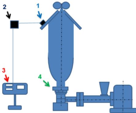
Fig. 1. The concept of application of Fuzzy Logic controller for automatic control of film thickness in the process of extrusion: 1 – film thickness sensor, 2 – measurand converter, 3 – control panel with Fuzzy Logic controller for film thickness adjustment, 4 – segmented cooling ring with automatic airflow regulation.
