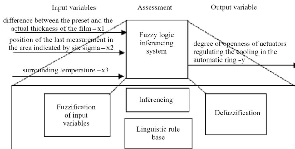
Fig. 4. Inferencing process based on fuzzy logic.
