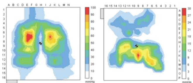
Fig. 3. Pressure maps – left pressure map from sensors on the chair seat, right: pressure map from sensors on the backrest [6].
