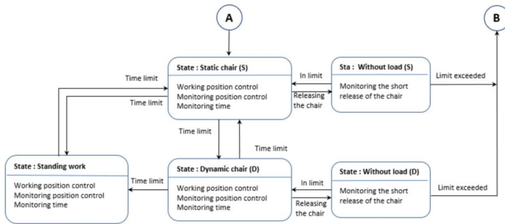
Fig. 5. The state diagram of ADW model – second part [authors].
