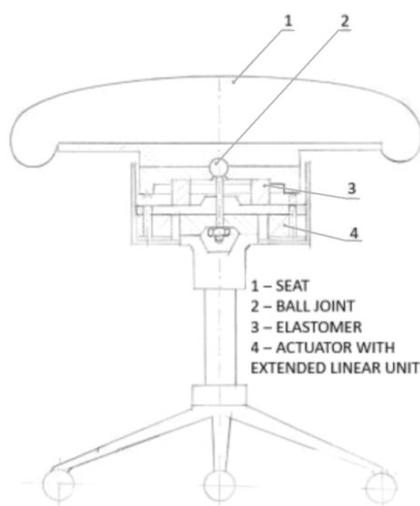
Fig. 2. Visualization of a possible design solution for automatic locking of the dynamic chair joint [authors].
