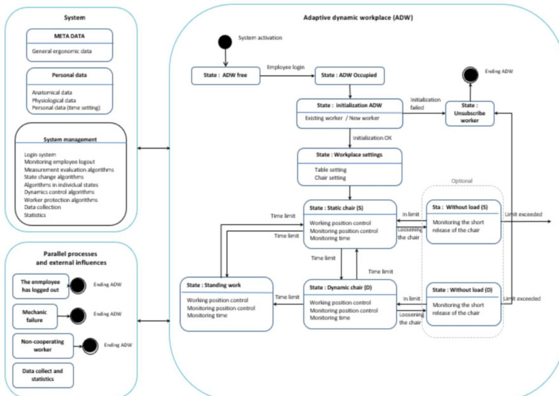
Fig. 6. The state diagram of the ADW model – parallel processes [authors].
