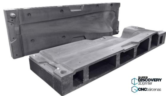
Fig. 4. 3D-printed two-part mold.
